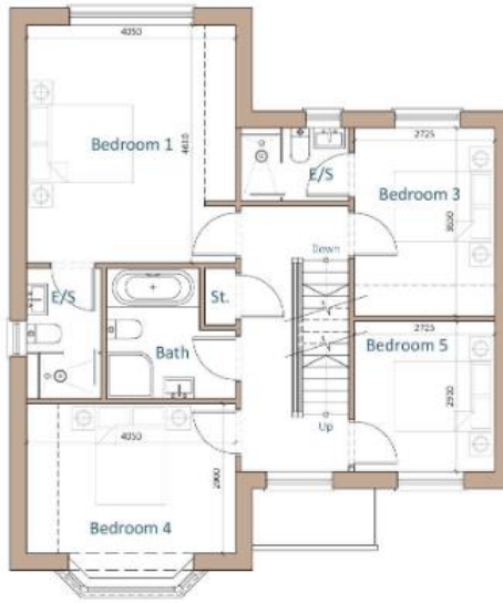
Proposed First Floor Plan Scale 1:50
